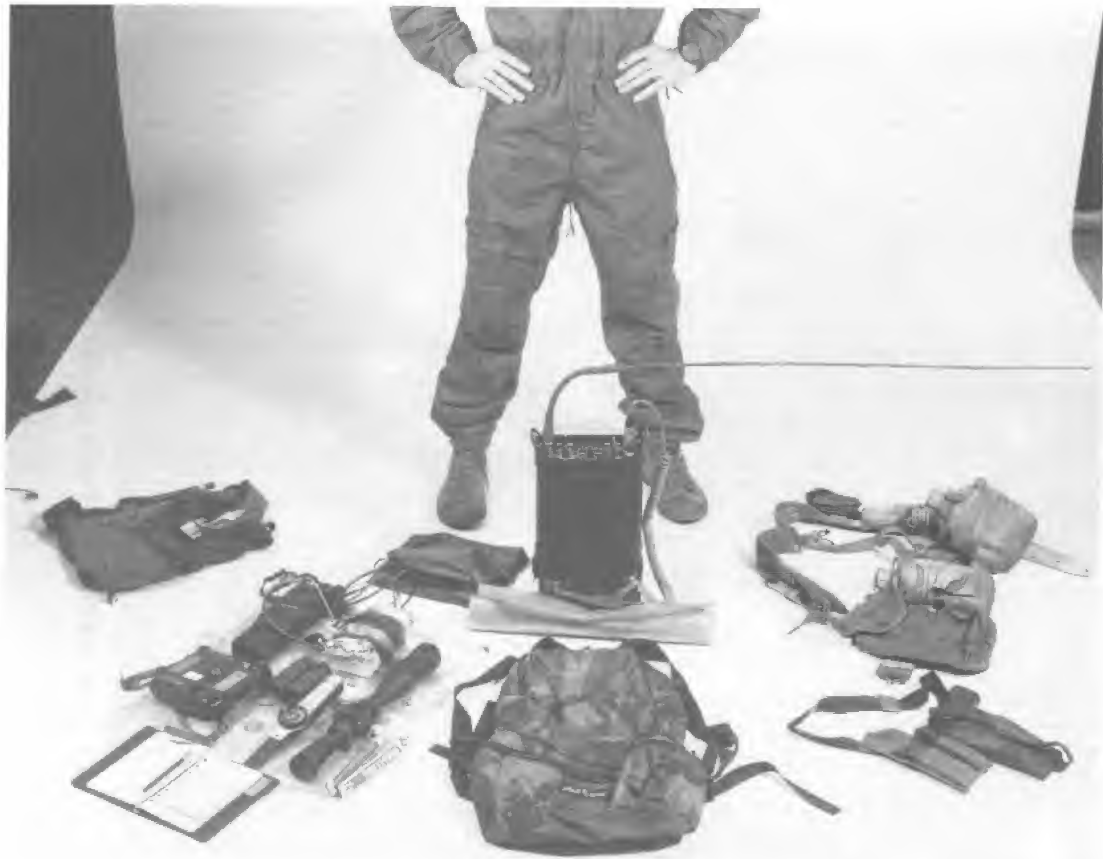
EQUIPMENT TO BE PREPPED FOR WATERBORNE INSERTION. NOTE THAT THE SCOPE HAS BEEN REMOVED FROM THE RIFLE AND WATERPROOFED; TORQUE WRENCH REQUIRED TO REMOUNT IN ORDER TO MAINTAIN ZERO.
